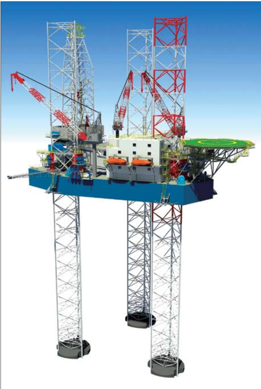
The KFELS B Class Bigfoot is equipped with larger spud cans for reduced bearings pressure and expands its operational coverage in more places, especially places where soft soil is predominant
