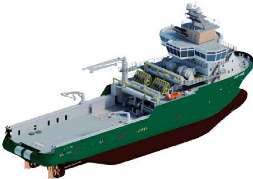
MTD 80210A, a large-sized AHTS measuring 88m in length and 22m in width, has a deadweight capacity of 3,500 metric tonnes and has tanks designed to carry drilling brine and marine gas oil
